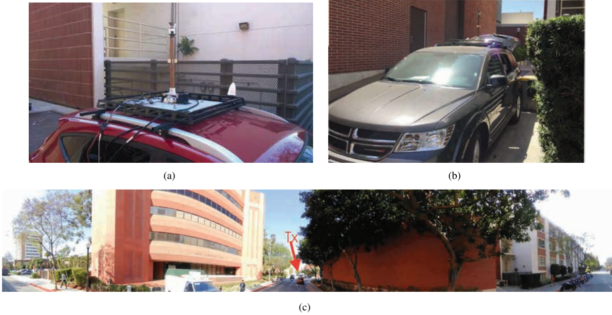
Fig. 6. Antenna arrays and measurement environments. (a) Antenna array on the Tx side. (b) Antenna array on the Rx side. (c) An example of the video shot on the RX side during the measurements.
